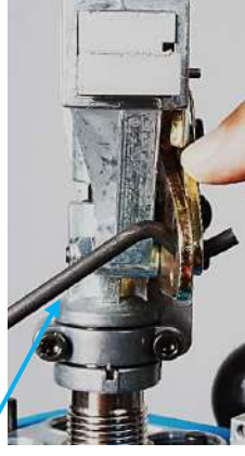
Slide Failsafe Rod out of Lock-Link Assembly
