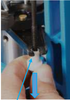
Pull Failsafe Bushing down out of Bracket
