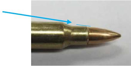
Taper Crimp of Rifle Cartridge with Cannelure
