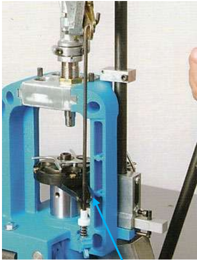
Align Failsafe Rod vertically with Failsafe Rod Bracket
