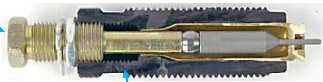
Rifle Size Die Body and Case— “sectioned”
