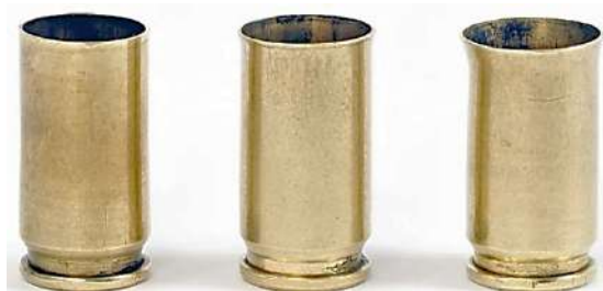
No Belling Adequate Belling Excessive Belling
