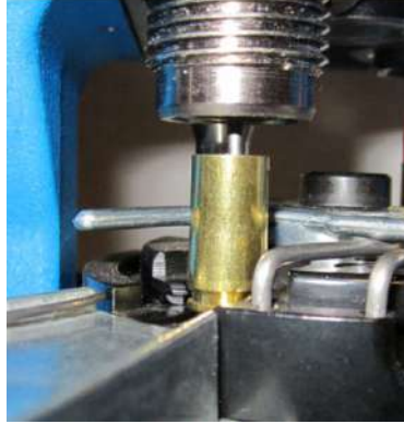
Station 1-Case entering Depriming/Sizing Die
