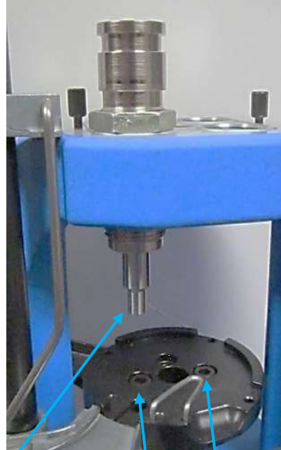
Two Platform Mounting Screws
