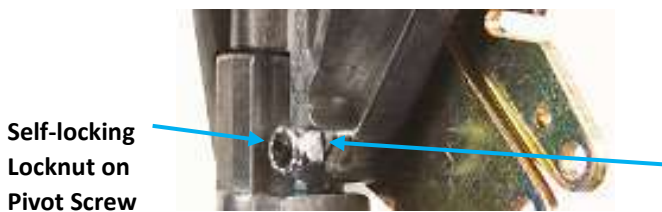
Loosen the Pivot Screw and Self-Locking Locknut on the back using a 7/16" wrench and a 5/32" Allen wrench
