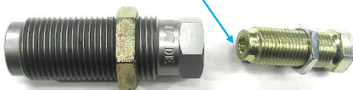
Bullet contacts edge of Seating Stem during Seating
