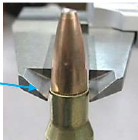
Crimp—reduce diameter no more than .001-.002"
