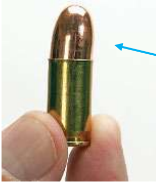
Just enough Belling to allow the bullet to sit in the case mouth without falling over and not shaving bullet material
