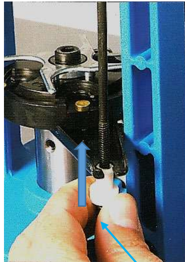
Push Failsafe Rod Bushing up into the Failsafe Rod Bracket
