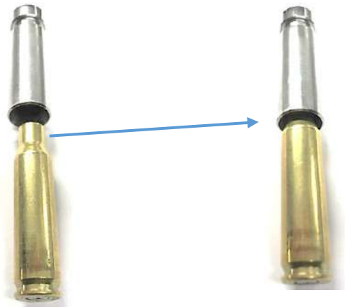
Rifle case neck fits up inside Caliber Specific Powder Funnel to Activate Powder Measure
