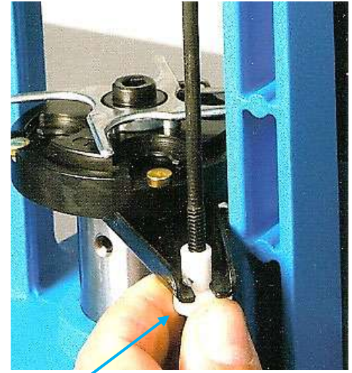
Push Failsafe Rod Bushing up into the Failsafe Rod Bracket
