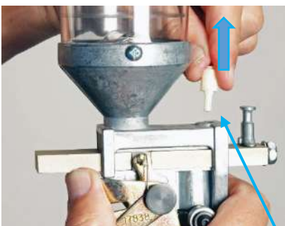
Remove the Retainer Plug and Slide the Powder Bar Spacer out
