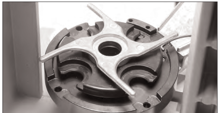
Figure 8 – This photo shows the index star in its proper position: the locating tabs centered in the shellplate.
