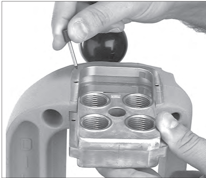
Figure 15 – Removing the toolhead.
