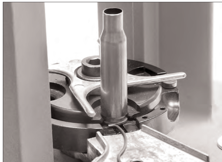
Figure 18 – Placing the cartridge case in the shellplate.
