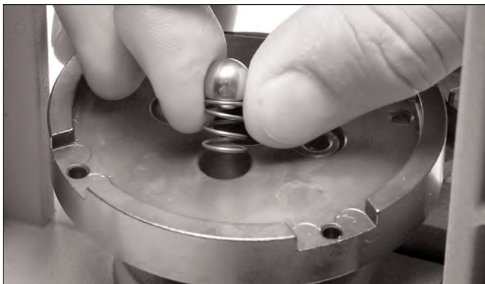
Figure 6 – This photo shows the index ball spring and index ball being placed in the platform.
