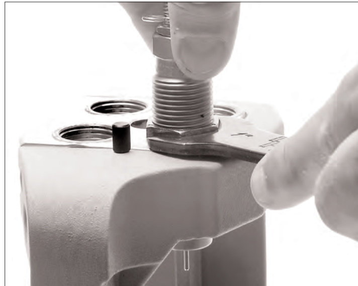
Figure 17 – Installing the sizing/decapping die in Station #1.
