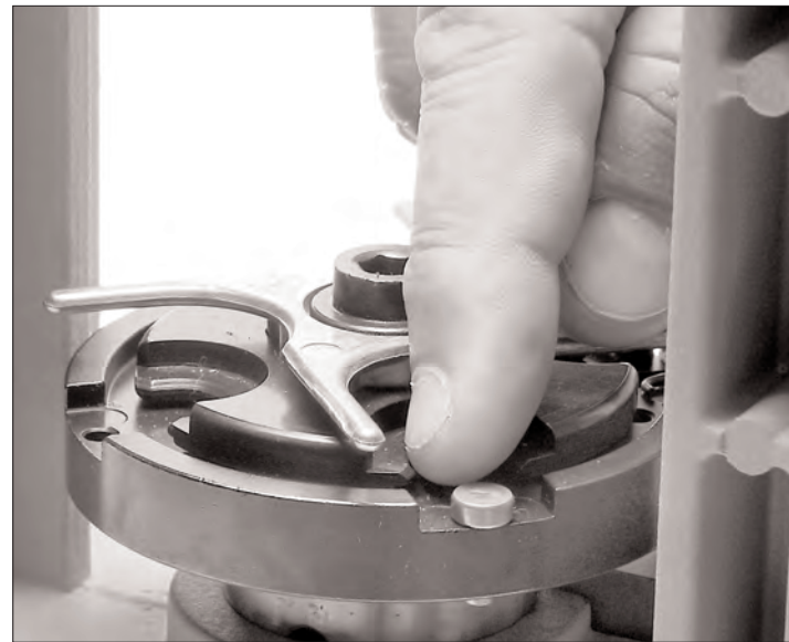
Figure 26 – Installing a brass locator button at Station #2.
