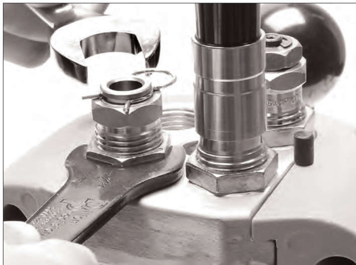
Figure 33 – Installing the bullet seating die in Station #3.
