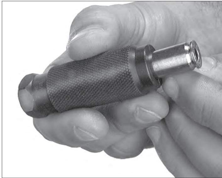
Figure 19 – Inserting a case in a case gage.
