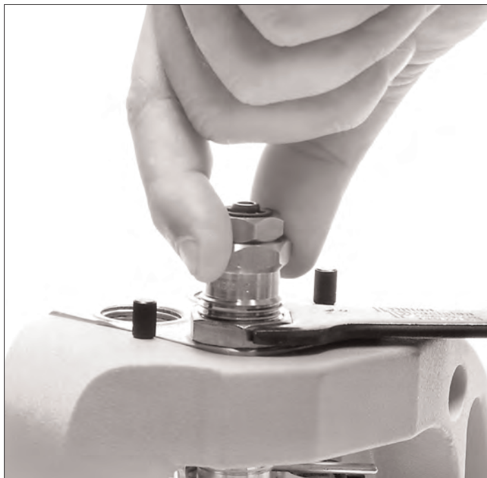
Figure 28 – Installing a sizing/decapping die in Station #1.
