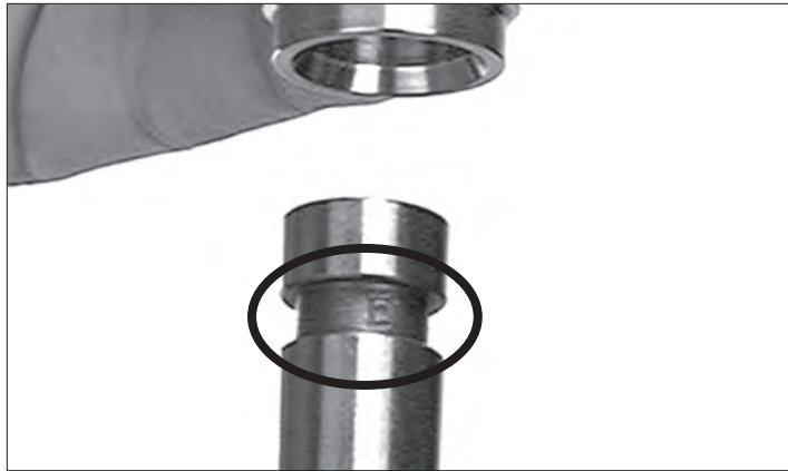
Figure 31 – The groove in the pistol powder funnel.
