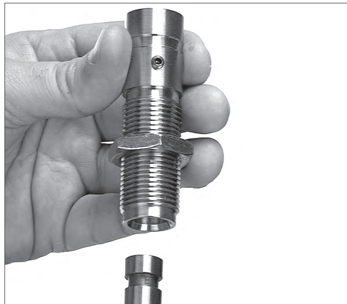
Figure 30 – Insert a pistol powder funnel into the powder die.
