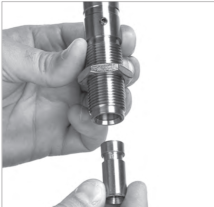
Figure 20 – Installing rifle powder funnel into the powder die.
