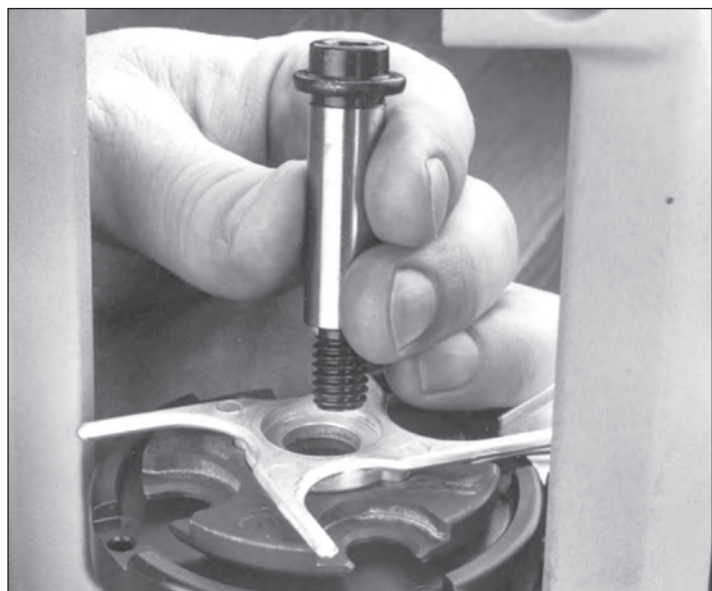
Figure 9 – Inserting the shellplate bolt, first through the index sprocket then the shellplate.
