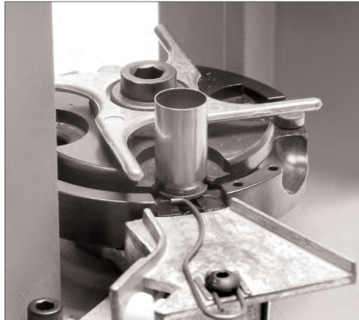
Figure 29 – Inserting an empty cartridge case in Station #1.
