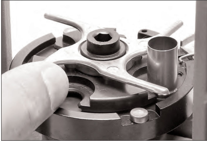
Figure 10 - This photo shows the proper method of indexing the shellplate and the proper installation of the locator buttons.
