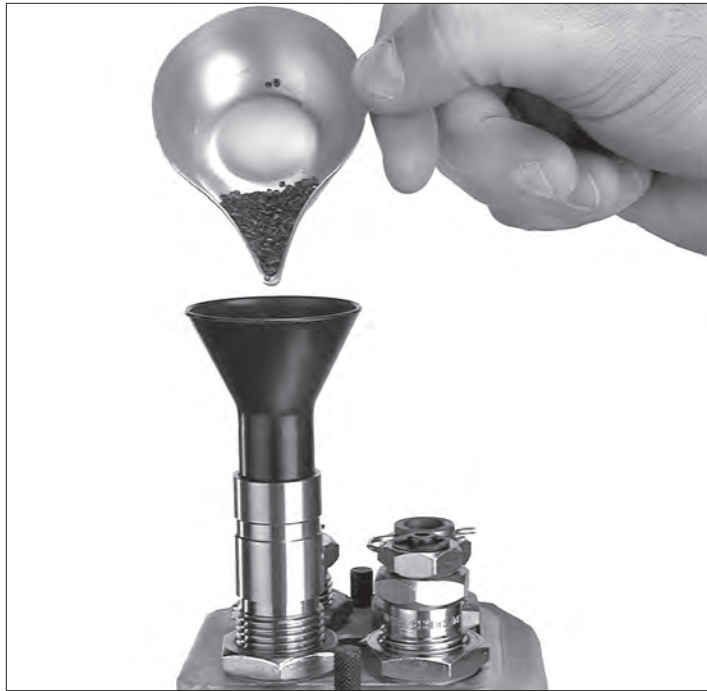
Figure 40 – Charging the case with powder at Station #2.
