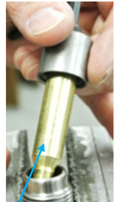
Place cap over drilled and tapped case and thread screw into case with the Allen wrench—“pulling” the case out of the die
