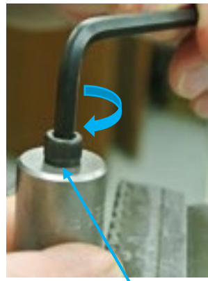
Place cap over drilled and tapped case and thread screw into case with the Allen wrench—“pulling” the case out of the die
