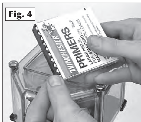
1. Fig #4 Slide the cardboard jacket back so that one half of the first row of primers is visible.
