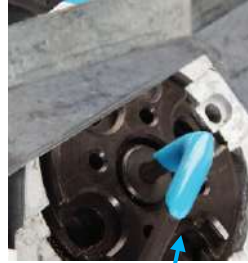
Remove Shellplate Bolt and Shellplate and store in the Conversion Box
