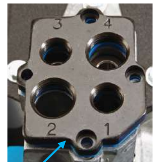
Place the Friction Plate on the Frame and then the Toolhead on the Friction Plate
