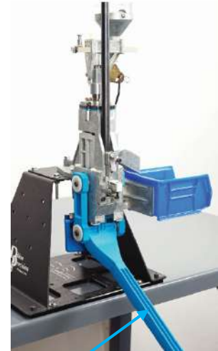
Station2--Case mouth flared and powder dispensed on the down stroke of the Operating Handle
