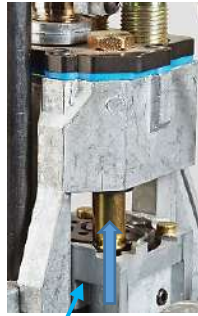
Station 1--Case entering Depriming/Sizing Die as the Operating Handle is lowered raising the Shaft/Shellplate
