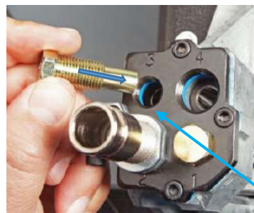
Thread Stem into Station #3 using the Bench Wrench or a 9/16” Wrench 5 turns down—further adjustment is required
