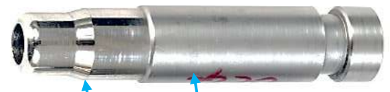
Station2--Case mouth flared and powder dispensed on the down stroke of the Operating Handle
