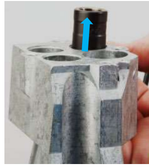
Remove the Crimp Die from Station #4
