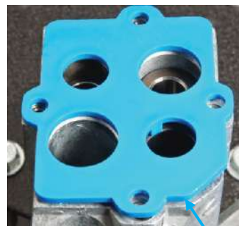
Place the Friction Plate on the Frame and then the Toolhead on the Friction Plate
