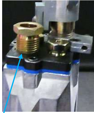
Install Universal Crimp Adjuster Plug in Station #4
