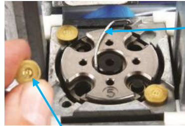
Install new Brass Locator Buttons from the Conversion Kit
