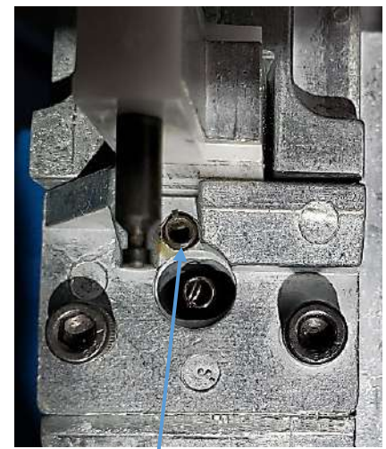
Forward Position Primer Slide Position Stop Set Screw
