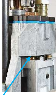
Station 1--Case entering Depriming/Sizing Die as the Operating Handle is lowered raising the Shaft/Shellplate
