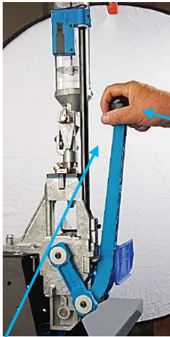
Station2--Primer seated push stroke of the Operating Handle from the at rest position
