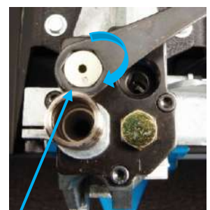
Thread Stem into Station #3 using the Bench Wrench or a 9/16” Wrench 5 turns down—further adjustment is required
