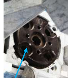
Remove Shellplate Bolt and Shellplate and store in the Conversion Box
