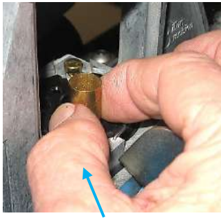
Station 1--Case manually inserted into Shellplate
