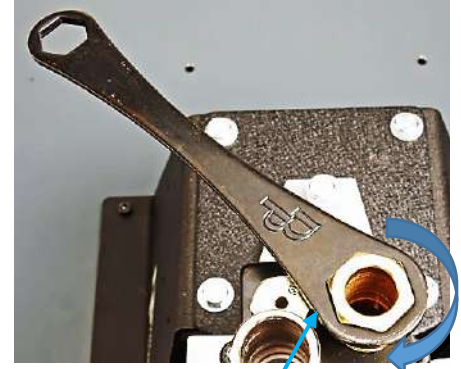
Thread Crimp Plug in 4 turns as a starting point
