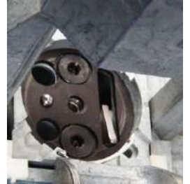
Clean the area under the Shellplate and the Index Ball and Spring
