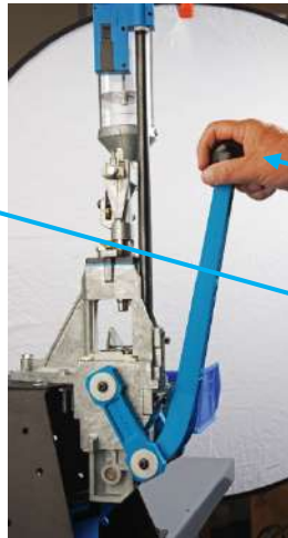
Station2--Primer seated push stroke of the Operating Handle from the at rest position
