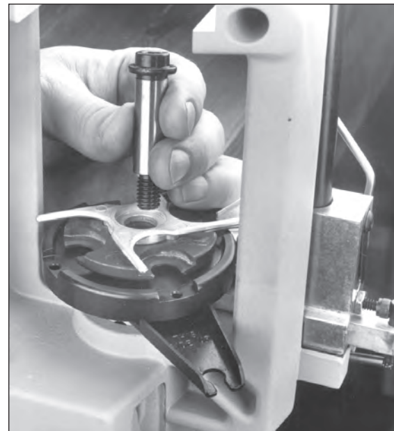
Fig. 8 - Inserting the shellplate bolt, first through the index sprocket then the shellplate.
