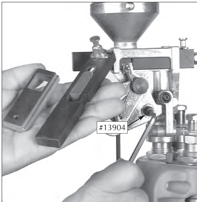
Fig. 24 - After emptying the powder measure, loosen the bellcrank screw (#13904) sufficiently to allow you to remove the powder bar. Insert the new powder bar and reverse this procedure.
