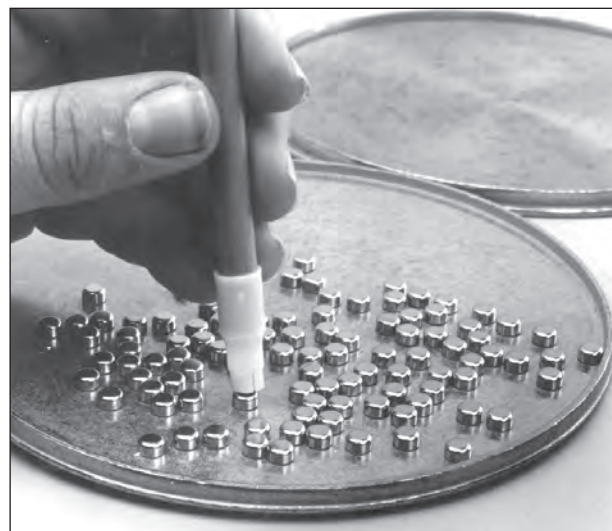
Fig. 25 - Use of the primer pickup tube and the Dillon Primer flip tray.
