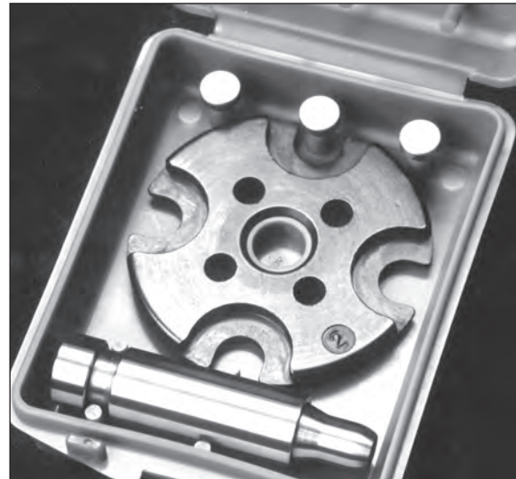
Fig. 4 - This photo shows a complete caliber conversion; the powder funnel, shellplate and locator buttons.
